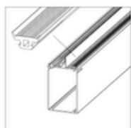
11. Side beam 1x sealing rubber
