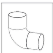
08. 90° rainwater discharge sleeve
