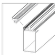
07A. End rafter 1x sealing rubber
