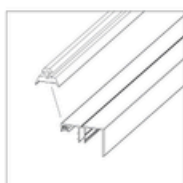
12. End cover strip 1x sealing rubber
