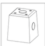
07. Concrete base with rainwater discharge (Option)
