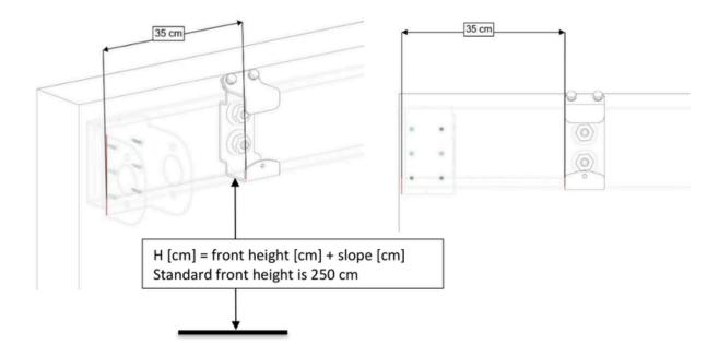
**2.** Fasten the brackets to the wall/ Use the correct hardware for your situation. We suggest to use minimum M12.
