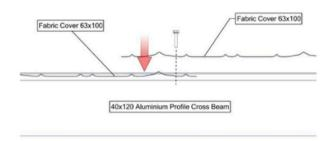
**4.** After installing the ceiling sheets, you can place the side cover profiles.
