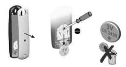
Using a small screwdriver loosen the screws on the reverse side of the remote control and remove the back cover.
